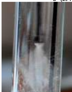
Fig. 2- Cavitating jet distribution pattern in a wave-guide with a spherical head in the distal part
